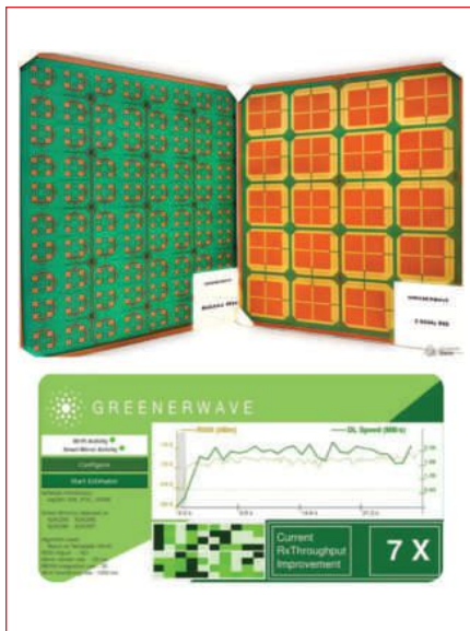
▲ Fig. 3 Greenerwave developed RIS for Wi-Fi to optimize the data transfer from an access point to a laptop, showing a 7x improvement back in 2016.
