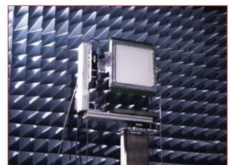
Fig. 7 Ka-Band transmit antenna prototype, which established a link with the Athena-Fidus GEO satellite.
